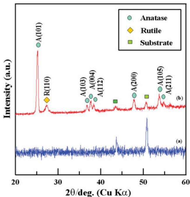
**Figure 5.** XRD patterns of AISI 304 stainless steel specimen (a) without and (b) with TiO<sub>2</sub> deposit. [Color figure can be viewed in the online issue, which is available at [www.interscience.wiley.com](http://www.interscience.wiley.com).]
