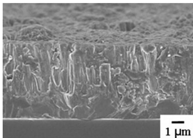
**Figure 4.** SEM cross-sectional morphology of TiO<sub>2</sub> film deposited for 1 h.
