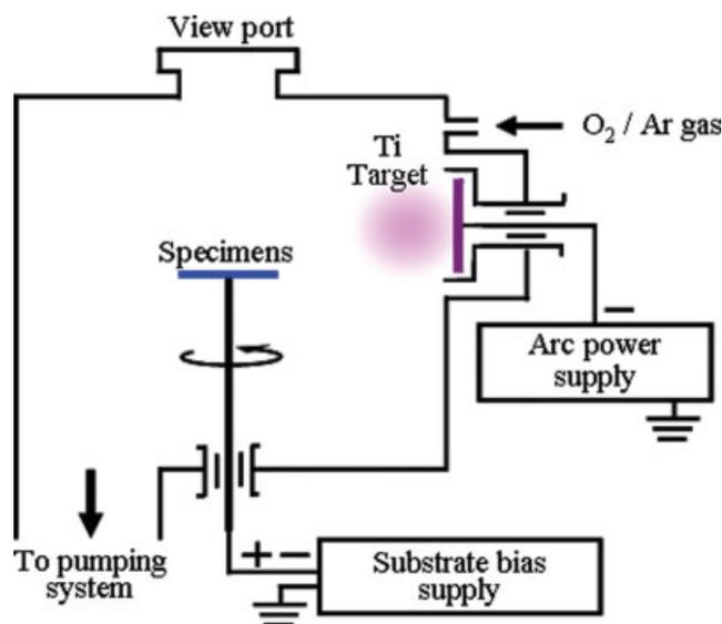
**Figure 1.** Schematic illustration of the AIP system. [Color figure can be viewed in the online issue, which is available at [www.interscience.wiley.com](http://www.interscience.wiley.com).]
