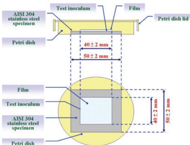
**Figure 3.** Test inoculum and film cover on the specimen. [Color figure can be viewed in the online issue, which is available at [www.interscience.wiley.com](http://www.interscience.wiley.com).]
