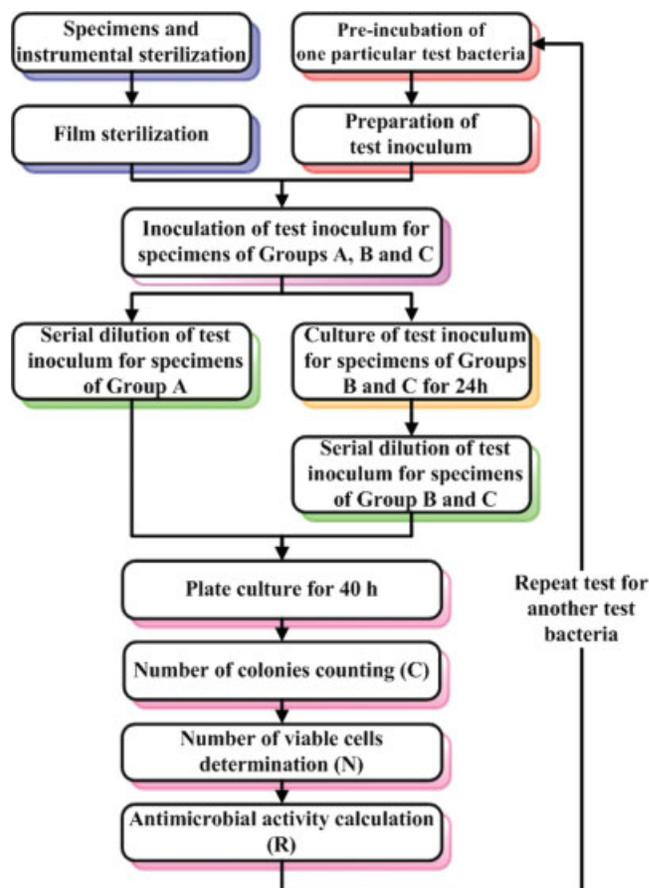
**Figure 2.** Antimicrobial test procedure according to JIS Z2801:2000. [Color figure can be viewed in the online issue, which is available at [www.interscience.wiley.com](http://www.interscience.wiley.com).]
