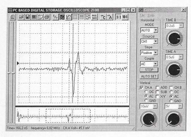
The resonance peak at 6.0 MHz is pushed up to the value of 8.4 MHz by the action potential of the firing axon (see also two maxima in graph 19). This frequency change is physically identical to a phase shift:
