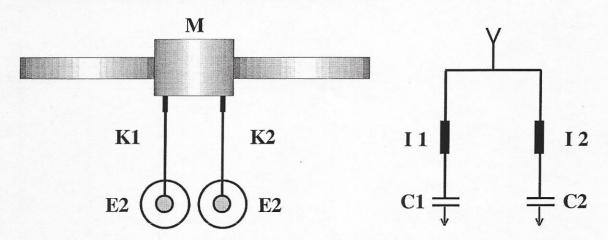
The metal wrist strap (M) of DE-KA-Titan ensures an optimal electrical skin contact. The wrist is capacitively coupled to other areas of the epidermis with the cables (K1 and K2) and the adhesive electrodes (E1 and E2). An oscillatory circuit is produced.
